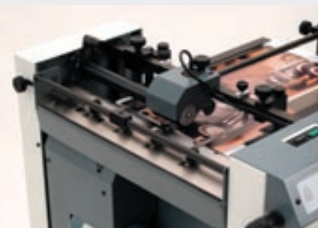
The sheet feeder with the special exit device.
