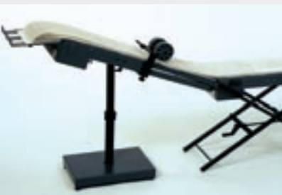
Another application sample. Transportation of processed material up to working height.
