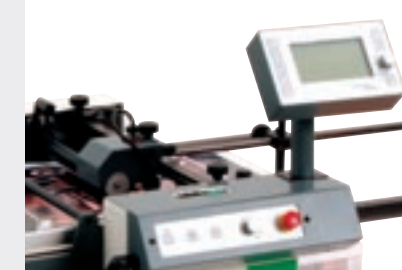
Control unit for counting, spacing and synchronising with the following machines.
