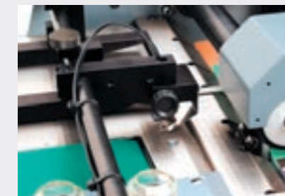
The sheet separation with integrated double sheet detection (optional).
