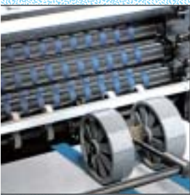
Steel-rubber rollers with diagonally toothed gears.
