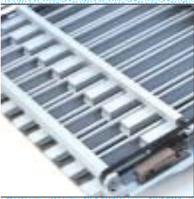
Detail of the automatic folding plate.
