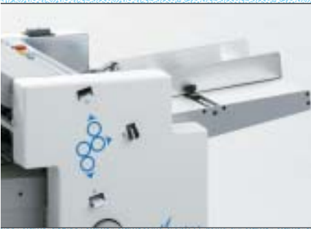
Friction feeder. For all A3-models.
